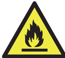
Caution: Risk of fire/ flammable materials
