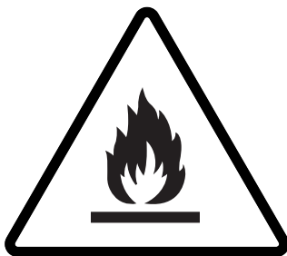
CAUTION: Risk of fire
