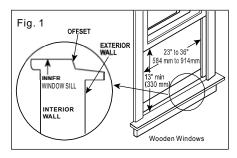
Lower sash must open sufficiently to allow a clear vertical opening of 13 inches (330mm). Side louvers and the rear of the AC must have clear air space to allow enough airflow through the condenser, for heat removal. The rear of the unit must be outdoors, not inside a building or garage.
