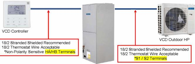
A) Complete VCD System + Proprietary Programmable VCD Controller
